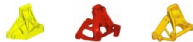
FIGURE 1. Optimization of Engine Mount Bracket
